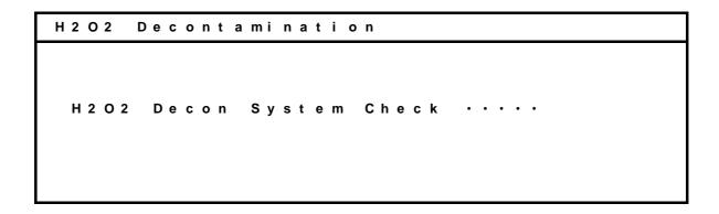
**7.** If the system is normal, the following display will appear. (If the system is not normal, refer to Table 2 on page 57.) Select OK and press the ENTER Key to start  $H_2O_2$  decontamination. Decontamination will be performed automatically to step 10. The buzzer will sound when decontamination has been completed (It takes about 1 hour 40 minutes after warming-up).
